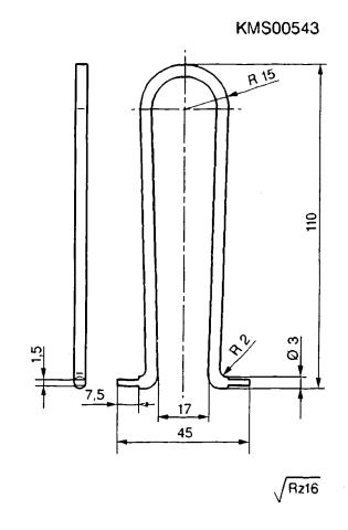
Driving-in mandrel for fitting excitation winding:
